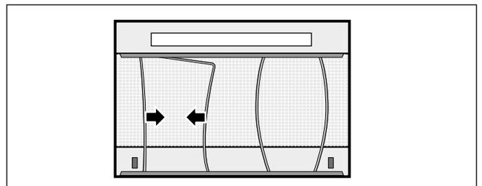
5. After removing the metal grease filter, clean the inside of the appliance.
