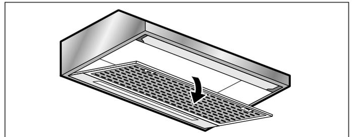
3. Position the filter grille at an angle and remove it.
