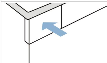
8. Pull out the condensation container horizontally and empty it.
