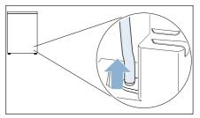
**Note:** The appliance comes delivered with the condensation hose already fitted to the connector.
