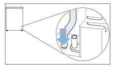
5. Take the drain hose from the accessories and push it fully onto the free connector.
