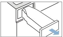
into the waste-water system via a drain hose 2. Pour out the condensation water.
