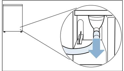
**Note:** The appliance comes delivered with the condensation hose already fitted to the socket.
