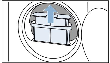
3. Remove the fluff from the fluff filter recess. Ensure that no fluff falls into the open shaft.
