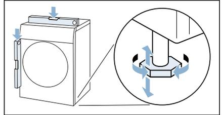
3. If necessary, turn the appliance feet to make sure it is level.
