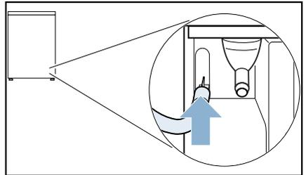
5. Take the drain hose from the accessories and attach it to the free socket, pushing it up to the stop.
