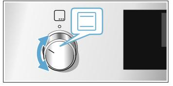
2. Use the temperature selector to set the temperature or grill setting.
