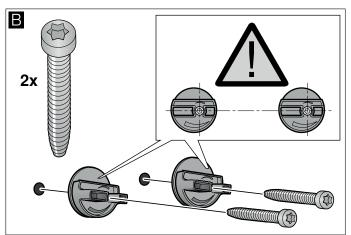
3. Screw in the threaded bolt, leaving it protruding out of the wall by 5–9 mm.
