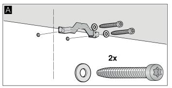
Screw on brackets for the extractor hood hand-tight. Do not firmly tighten the screws.
