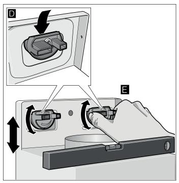
Firmly tighten the screws for the brackets. When doing so, hold the brackets securely in place.
