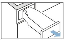
2. Push the condensation container back into the appliance until you feel it lock into place.
