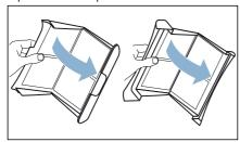
Remove all fluff from both parts of the filter.
