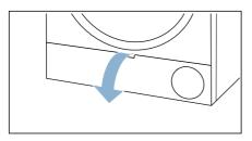
3. Unlock the levers on the heat exchanger cover.
