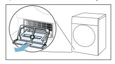
c) Rinse the insert under running water and dry it off.
