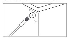
3. Reconnect the hose at the rear of the appliance and check for leaks.
