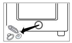
3. Put the pump cover back in place and screw it back on fully.
