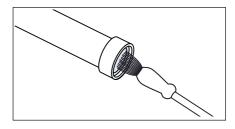
3. Connect the hose and check for leaks.
