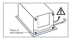
Push the bottom plate onto the underside of the appliance and screw it in place.
