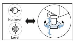
**Note:** If the appliance is ever moved, check that it is still level and re-level it if necessary.
