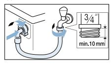
2. Carefully turn on the taps and check that there are no leaks.
