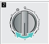
To use the small hotplate again, turn the control knob anticlockwise to position 0 and then switch the hotplate on again.
