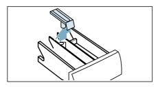
Clean the detergent dispenser tray and insert with water and a brush, and dry it. Clean the inside of the housing as well.
