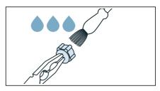
Connect the hose and check for leaks.
