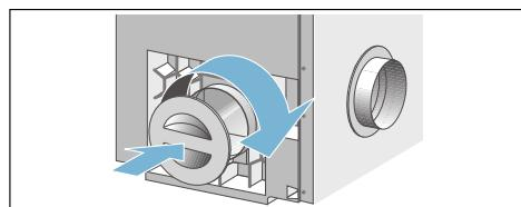
**Note:** If there is a high level of condensation in the exhaust air duct, it is advisable to fix a condensation collector (standard) or a drain hole with a diameter of approximately 3 mm to the lowest part of the exhaust air duct.
