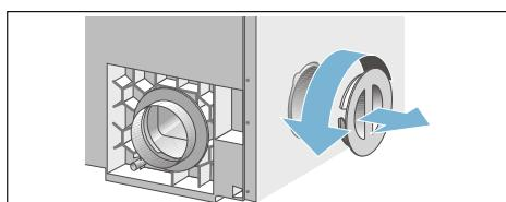
2. Remove the bayonet ring from the back panel and attach it to the opening on the side panel.
