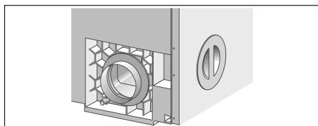
The exhaust air opening on the back panel is open when the dryer is delivered (bayonet ring). The exhaust air opening on the left side panel is sealed with a cover.
