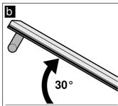
Lift the oven door slightly and pull it out.
