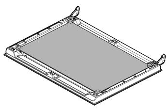
**Note:** The middle panel is kept in place with rubber bushings rather than retaining pins.
