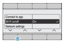
Use either of the right-hand arrow buttons on or off to switch Wi-Fi on or off.
