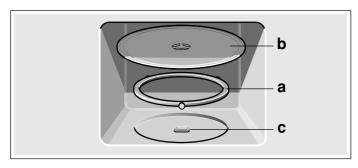
**Note:** Never use the appliance without the turntable. Make sure that it is properly engaged. The turntable can turn clockwise or anti-clockwise.
