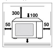
The appliance is ready to be plugged in and may only be connected to an earthed socket that has been correctly installed. The circuit breaker must have a rating of 12 A (L- or B-type circuit breaker). The mains voltage must correspond to the voltage specified on the rating plate.
