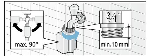
**Note:** Turn on the tap carefully, checking the leak tightness of the connection points. The screw connection is under mains water pressure.
