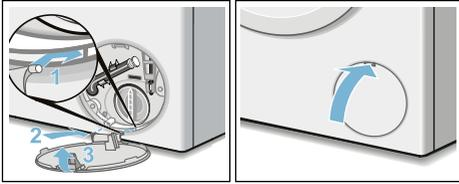
**Note:** To prevent unused detergent from flowing straight into the drain during the next wash, pour 1 litre of water into compartment
