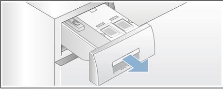
b) Pull the catch (A) on the back of the drawer handle (in the centre at the bottom) slightly towards you. This unlocks the drawer handle (B), which you can then pull off by lifting it upwards.
