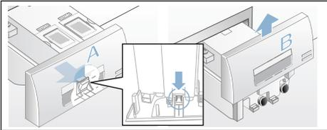
c) To empty the dispensers, carefully pull off each of the sealing plugs and empty the contents into a suitable container.
