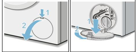
4. Take the drain hose out of the retainer. Remove the sealing cap and pour the water out into a suitable container. Replace the sealing cap and place the drain hose back in the retainer.
