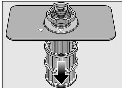
3. Remove any residue and clean filters under running water.
