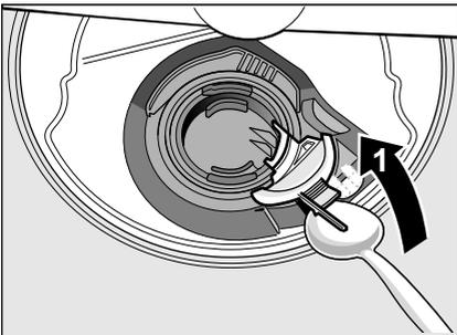
6. Check impeller wheel and remove any foreign objects.
