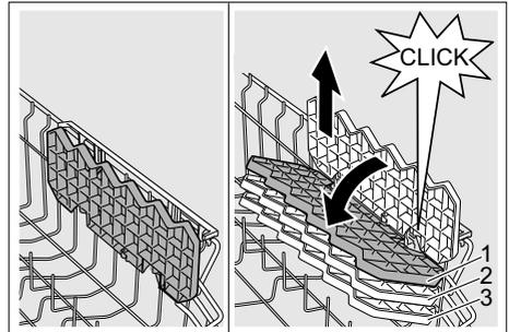
\* Depending on the model, a 3-fold height adjustment is possible. To do this, first place the etageres vertically and pull up, then place at a slight angle, push down to the required height (1, 2, or 3) and snap into place.
