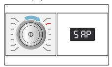
Press (Start/Pause) D to connect to the network. will flash on the display.
