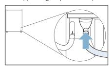
**6.** Secure the other end of the drain hose in place using the remaining accessories (depending on the connection type).
