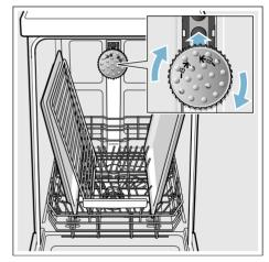
To ensure that the spray jet can reach all parts, arrange the baking sheets as illustrated (max. 2 baking sheets and 2 arilles).
