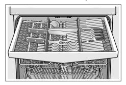
Depending on the features of your dishwasher, you can fold down the side shelves to provide more room for taller items of cutlery. The front rows of prongs can be folded down to provide room for wider handles.
