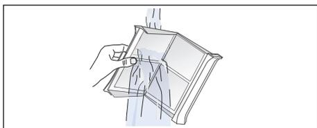
7. Dry the fluff filter, close it and reinsert the two-part fluff filter.
