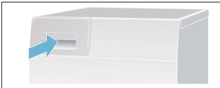
**Note:** The filter in the condensate container filters the condensation which is used during the dryer's automatic cleaning cycle. The filter is cleaned by emptying the condensation. Nevertheless, you should check the filter regularly for remaining deposits and remove them. See → Page 32.
