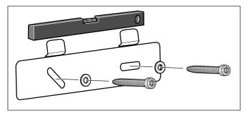
2. Screw in the threaded bolt, leaving it protruding out of the wall by 5 - 9 mm.
