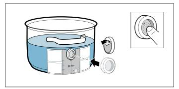
Press down all over the surface of the silicone patch, including in the centre.
