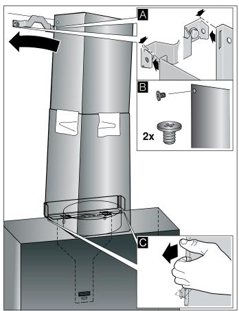
Clip the lower flue duct section in at the retaining bracket. The connection cable must not be damaged.
