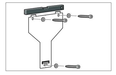
Screw in the mounting supports for the extractor hood until they are hand-tight, use a spirit level to level the appliance and then screw the mounting supports in fully.
