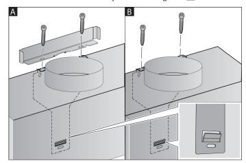
5. If no duct is to be fitted, screw in the two locking screws without the bracket.
