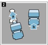
3. Use the hook to attach the rear holder into the upper hole **a** and push it into the lower hole **b** (fig. **3**).
