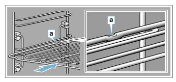
When inserting baking trays, ensure that the catch tappet **a** is at the rear and is facing downwards. The sloping edge of the accessory **b** must be facing forwards towards the appliance door.
