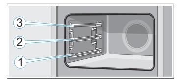
When using positions 1, 2 and 3, always insert the accessory between the two guide rods for a shelf position.
