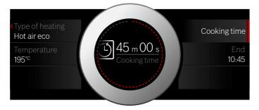
**4.** Press the ▷ Start/Stop button to start. The cooking time counts down.
