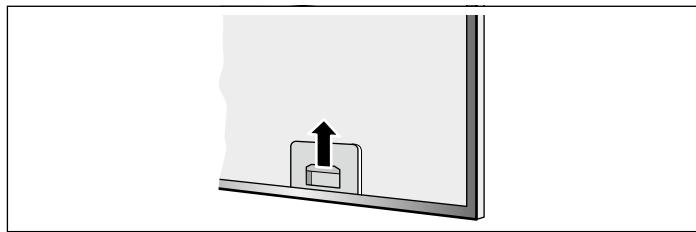
1. Open the lock on the metal grease filters and remove the filters from the retainer.
