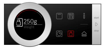
6. Press the start/stop button ▷ to start. The cooking time counts down on the display.
