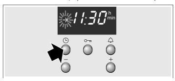
**6.** Use the + button to set a later end time. The setting is adopted after a few seconds. The display shows the end time until the oven starts operating.
