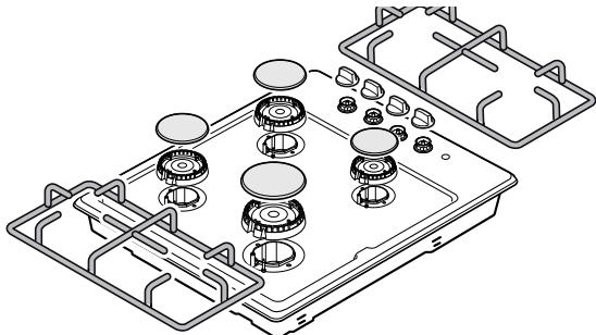
2. Loosen the hob plate burner connection screws.
