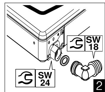
If liquid gas (LPG) is used, the gas connection should be established via a gas hose or a fixed connection.
