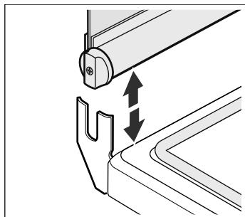
The glass cover must be completely open when removing the glass panel to clean it or to tighten the hinges.
