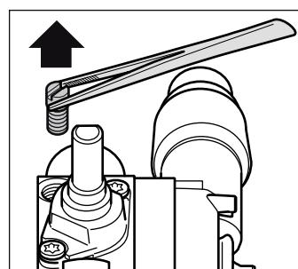
2. Select the appropriate new bypass nozzles from the table in accordance with the gas type to which you are converting. See the section "Technical data – Gas".
