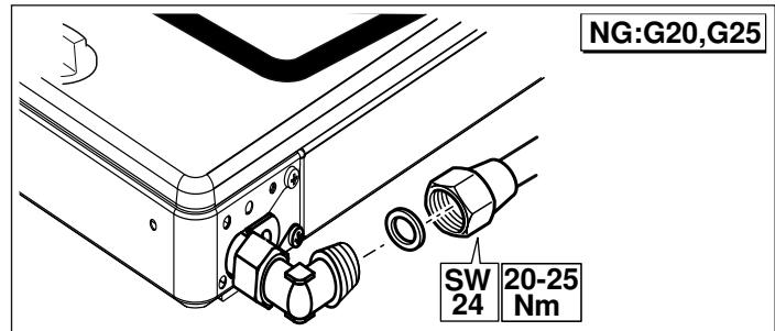
**Note:** If a cylindrical connection is required, replace the clamp that is installed at the factory with the cylindrical clamp from the accessory kit.
