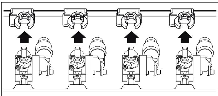
The bypass nozzles must then be tightened as far as they will go.
