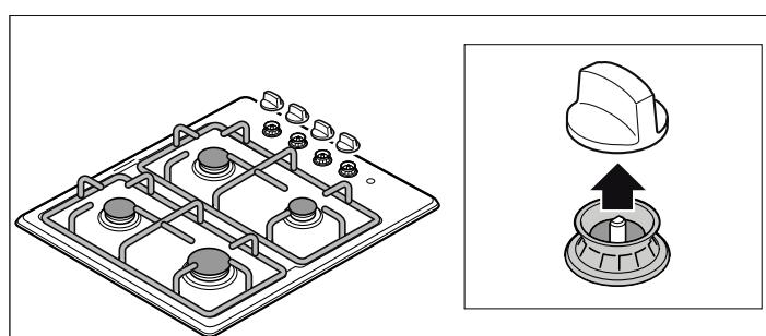
**Adjust the bypass nozzles for the conversion from natural gas to liquid gas, or replace these:**
