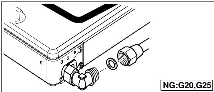
Place the gas pipe or the flexible safety gas hose with thread (using a size 24 key) and with a new seal on the connecting piece and tighten it securely.
