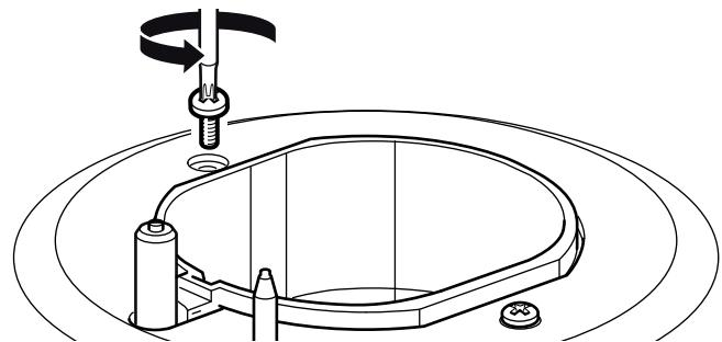
3. For models with electric hotplate (optional): After loosening the burner screws, turn the hob over and remove the connection nut for the electric hotplate.
