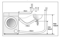
**Note:** If the hose holders are used, the possible hose lengths are reduced!
