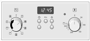
Use the temperature selector to set the temperature or the grill setting.
