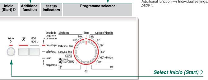
Programme selector for switching the machine on and off and for selecting the programme. Can be turned in either direction.
