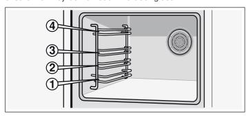
When the accessories are pulled approximately halfway out, they lock into position. This allows meals to be taken out easily.
