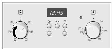
2. Use the temperature selector to set the temperature or the grill setting.
