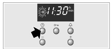
**6.** Use the + button to set a later end time. The setting is adopted after a few seconds. The display shows the end time until the oven starts operating.
