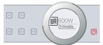
The microwave output and a default cooking time are shown in the display. The  $\bigcirc$  field lights up red.
