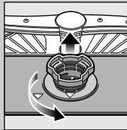
Rotate filter cylinder, remove filter system ...
