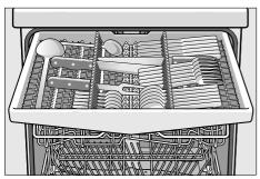
Depending on the model, you can fold down the side shelves to provide more room for taller items of cutlery. The front rows of prongs can be folded down to provide room for wider handles.
