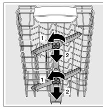
**3.** Remove the lower spray arm 24 upwards.
