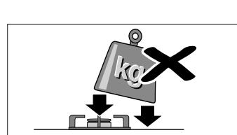
Place the pans on the pan supports, never directly on the burner.
