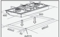
Please perform the tapping on the countertop according to the tapping template (keeping to the installation size of all the five types of products). To ensure the proper connection of the gas hose, a space of at least 100mm height should be kept available below the gas hob.
