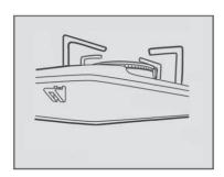
Follow the method shown in the illustration on the left and clamp the four spring sheets supplied with the product to the corresponding four installation positions on the back shell.
