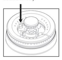
After cleaning is complete, please re-install the support, burner heads and caps in accordance with the illustration (page 10). Any permanent scratches on the top sheet surface caused by incorrect installation are not covered by the warranty.
