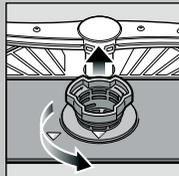
Rotate filter cylinder, remove filter system ...
