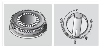
Outer flame on minimum, inner flame on full power.
