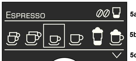
The status line **5a** in the display **5** shows the name of the type of drink, along with the strength setting, e.g.  $\textcircled{0}$  and per-cup quantity, e.g.  $\square$ . The selection line **5b** shows symbols for drink selection.
