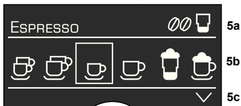
The status line **5a** in the display **5** shows the name of the type of drink, along with the strength setting, e.g. *00* and per-cup quantity, e.g.
