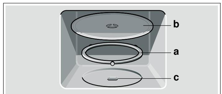
**Note:** Do not use the appliance if the turntable is not in place. Ensure that it is properly slotted into place. The turntable can turn clockwise or anti-clockwise.
