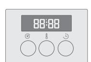
The LED display shows the data of programme which could to be set alternately before the programme starts, such as start in time, washing temperature, spin speed, etc; only remaining time is displayed after the programme starts.
