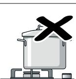
Always centre the pan over the burner, not to one side. Otherwise it could tip over.
