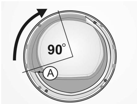
**13.** Note the new position of the cover glass. The leading edge of the raised glass edge should have moved 90 degrees clockwise from its starting point as shown in the illustration below as (A).
