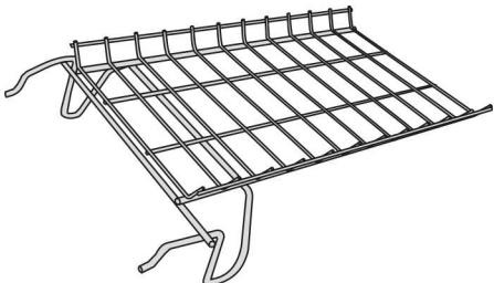
3. Hold the dryer rack by the center section as shown below and insert it horizontally all the way into the drum. Then bring it back towards the front and align the forward ends with the two holes beside the lint filter.
