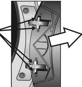
Avoid allowing the 4 plastic bushings to fall off the hinge pins. If any of the bushings do fall off, reinstall them on the hinge pins prior to reinstalling the door.
