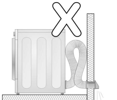
Do not allow exhaust ductwork to be longer than necessary. Longer ductwork will reduce airflow and will result in longer drying times.
