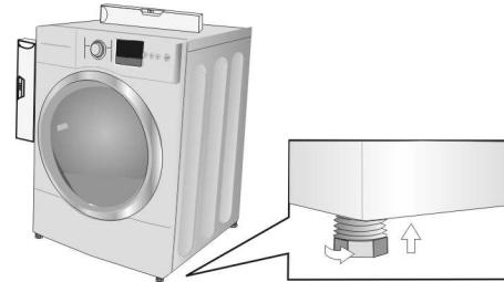
The dryer should be level with all four feet firmly on the ground. The dryer must not wobble. If the dryer is not level or if it does wobble, the feet must be adjusted. Adjust the height-adjustable feet using the 1 in. (25mm) wrench until the dryer does not rock and is level, both front-to-back and side-to-side.
