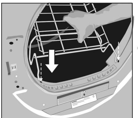
4. With the forward ends engaged in the holes, lower the back of the rack so that it sits in place, braced against the inner surface of the dryer housing.
