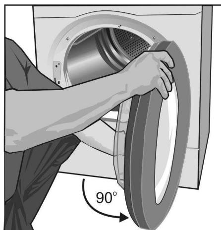
**9.** Remove the four screws holding the front ring to the door body.
