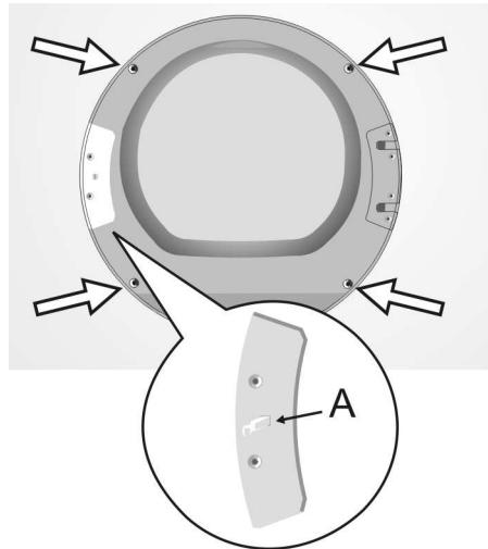
**20.** Remove the two screws holding the plastic cover plate over the left hand hinge mounting position on the dryer housing. Remove the plate and set it aside with the two screws.
