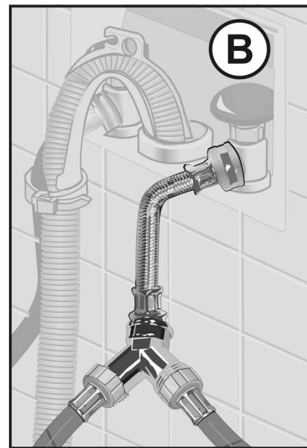
4. Attach the short hose to the cold water faucet. Tighten the connection by hand until the coupling is seated on the faucet.
