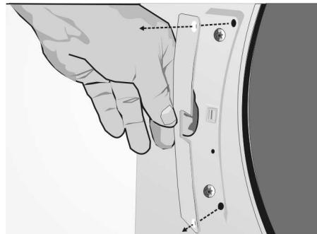
**21.** Remove the two screws holding the metal door hinge to the dryer housing. Remove the hinge from the housing.
