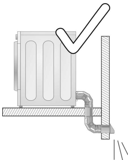
Do not allow exhaust ductwork to be crushed or otherwise constricted. Constricted ductwork will reduce airflow and result in longer drying times. Constricted ductwork could reduce exhaust airflow enough to cause an error condition, halting the dryer cycle. Check to be sure the exhaust duct is not crushed or constricted.
