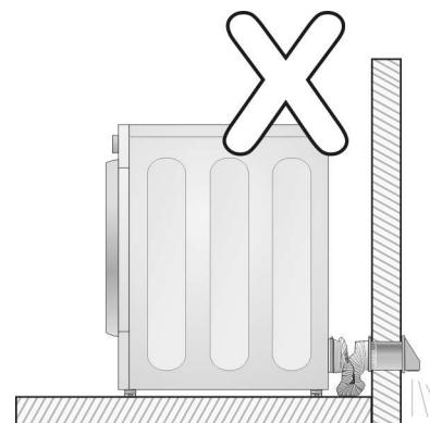
Keep exhaust ductwork as short and as straight as practical. This will increase air flow and result in shorter drying times.
