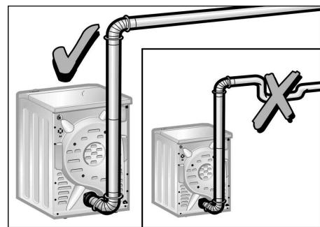
Exhaust ducting which is longer than specified in the maximum ductwork length table on page 18 is not permitted. Not adhering to this table will extend drying time, cause lint to accumulate and affect dryer performance and life-time.
