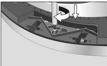
**18.** Rotate the striker cover and striker 180 degrees so the assembly fits to the install area on the opposite side of the door (where the hinge had been). Reinstall the striker cover and striker to the new location and securely tighten the two cover screws.
