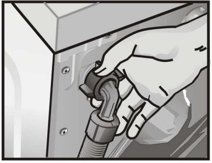
Attach the dryer water supply hose to a cold water faucet (the faucet must be located within 4 ft (1.2 m) of the water inlet valve on the back of the dryer).
