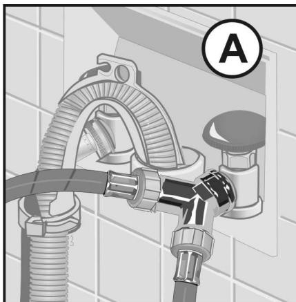
2. Check to be sure that the rubber washer is fully inserted and seated in the female end of the short hose prior to continuing. The rubber washer is shown as item 3 in the
