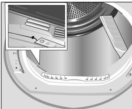
This deposit can easily be removed by wiping the sensors (the two bars next to the lint filter) with a cloth and a little white vinegar.
