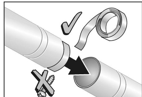
All joints should be tight to avoid leaks. The male end of each duct section must point away from the dryer.
