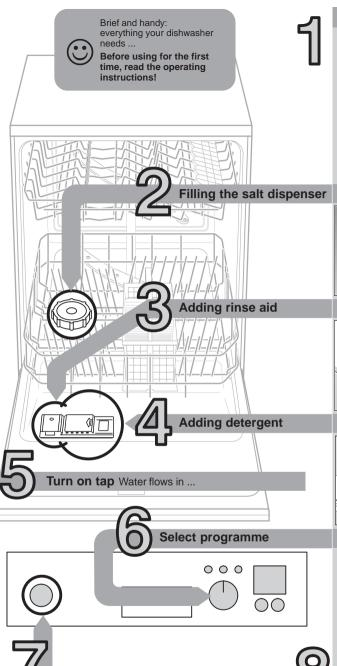
Switch on the appliance Here we go ... Press main switch, running time of the selected
