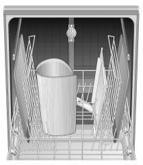
Large sheets or grilles and plates which have a diameter greater than 30 cm (gourmet plates, pasta plates, dinner plates) can be cleaned with the aid of the spray head. To do this, remove the top basket and insert the spray head as illustrated in the diagram.
