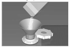
The LOW SALT indicator 7 on the front panel will light up initially but will extinguish again after a short period when the salt solution has become sufficiently concentrated.
