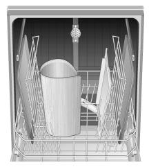
Large sheets or grilles and plates which have a diameter greater than 30 cm (gourmet plates, pasta plates, dinner plates) can be cleaned with the aid of the spray head. To do this, remove the top basket and insert the spray head as illustrated in the diagram.
