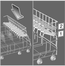
The cup shelf can be inserted into either position 1 or 2 as shown in diagram.
