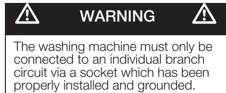
The household electrical voltage must correspond to the voltage specification on the washing machine (rating plate, see page 20).
