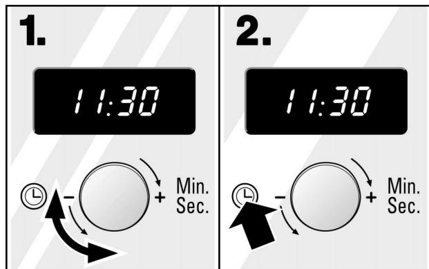
1. Set the time using the rotary knob. 2. Press the clock button.
