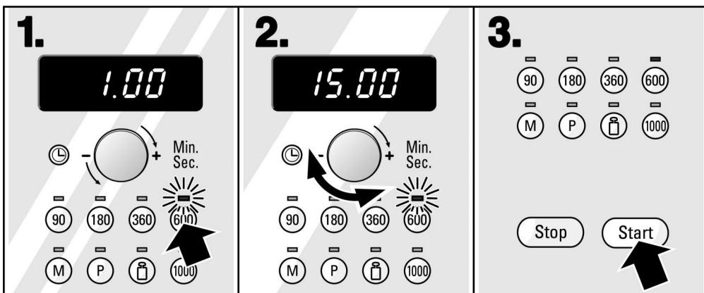
1. Press the button for the microwave setting you require. The indicator light above the button flashes.
