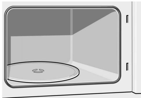
You should only use the appliance with the turntable in place. Ensure that the support ring is properly fitted. The turntable can turn anti-clockwise or clockwise.
